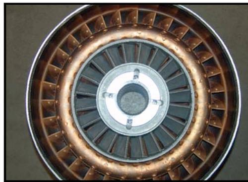
Located above is the impeller with a green tag. The impeller to the far left is designated by an orange tag and located directly left an impeller with a black tag. Note the number and angle of the primary fins and stator fins.
