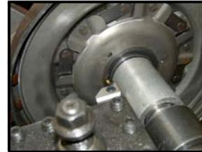
Notice the machining accomplished using a .060 grooving tool.
